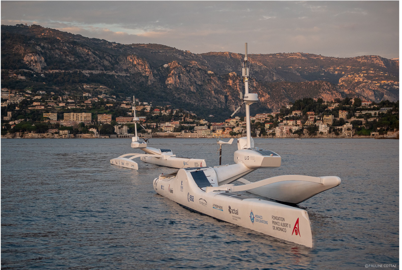
Drone 'Sphyrna' S70 (21m) and S55 (17m) in Villefranche Bay, for acoustic acquisition of cetacean signals during the Sphyrna Odyssey 2019-2020 mission.
