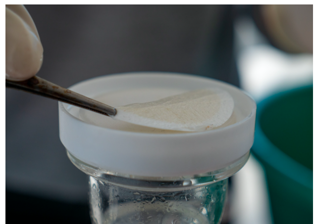
Figure 30. Extraction of eDNA by seawater filtration, performed during the Sphyrna Odyssey 2020 mission by Sara. The eDNA was obtained by filtering a volume of sea water through filters (porosity 0.45 \mu\text{m} )
