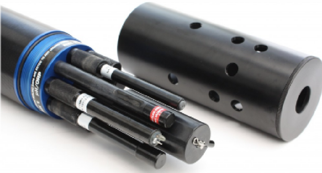
Figure 35. Multiparameter chemical probe (Aquaread AP-7000), with sensors included in Sphyrna ( https://www.aquaread.com/portofolio/ap-7000/ ).
