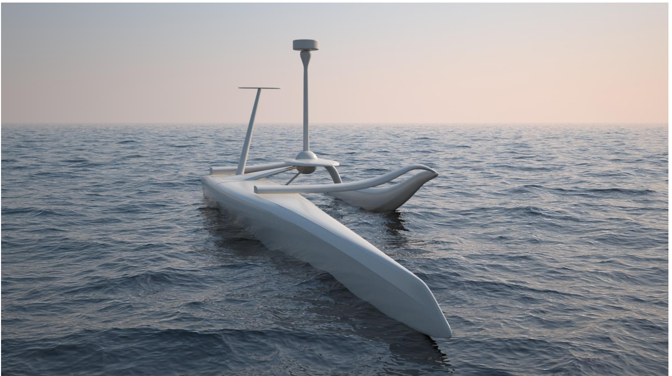
Figure 28. Computer-generated image of the S24 drone (6m20), front view (actual size). Design completed, production scheduled for July-August.
