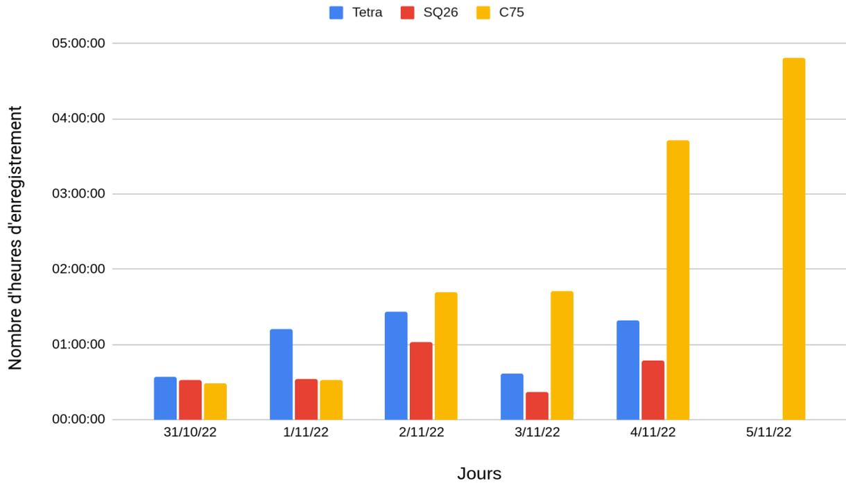
**Figure 5.1:** Graph representing the acoustic acquisition effort (number of hours) for the 3 antennas deployed from the IsbjornII, per day following the three types of measurements: antenna of 4 SQ26 hydrophones (Tetra), or single SQ26 hydrophone at 60 kHz bandwidth or C55 broadband alone.
