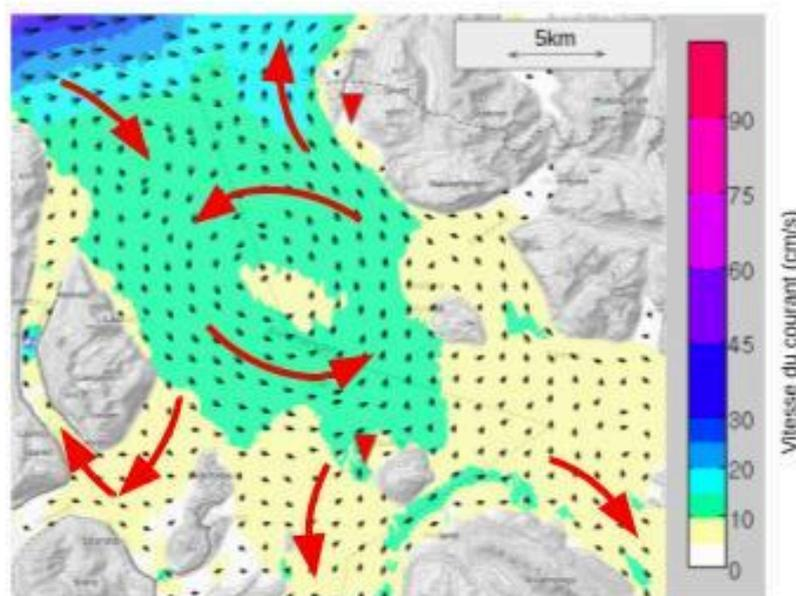
**Figure 3.3** : Zoom on the nature of the average currents off Seglvik (red triangle to the North) and location of the 2 long-term acoustic stations installed by our mission, for 3 months of recording with our systems (▲). The distance between the two antennas is approximately 18 km.
