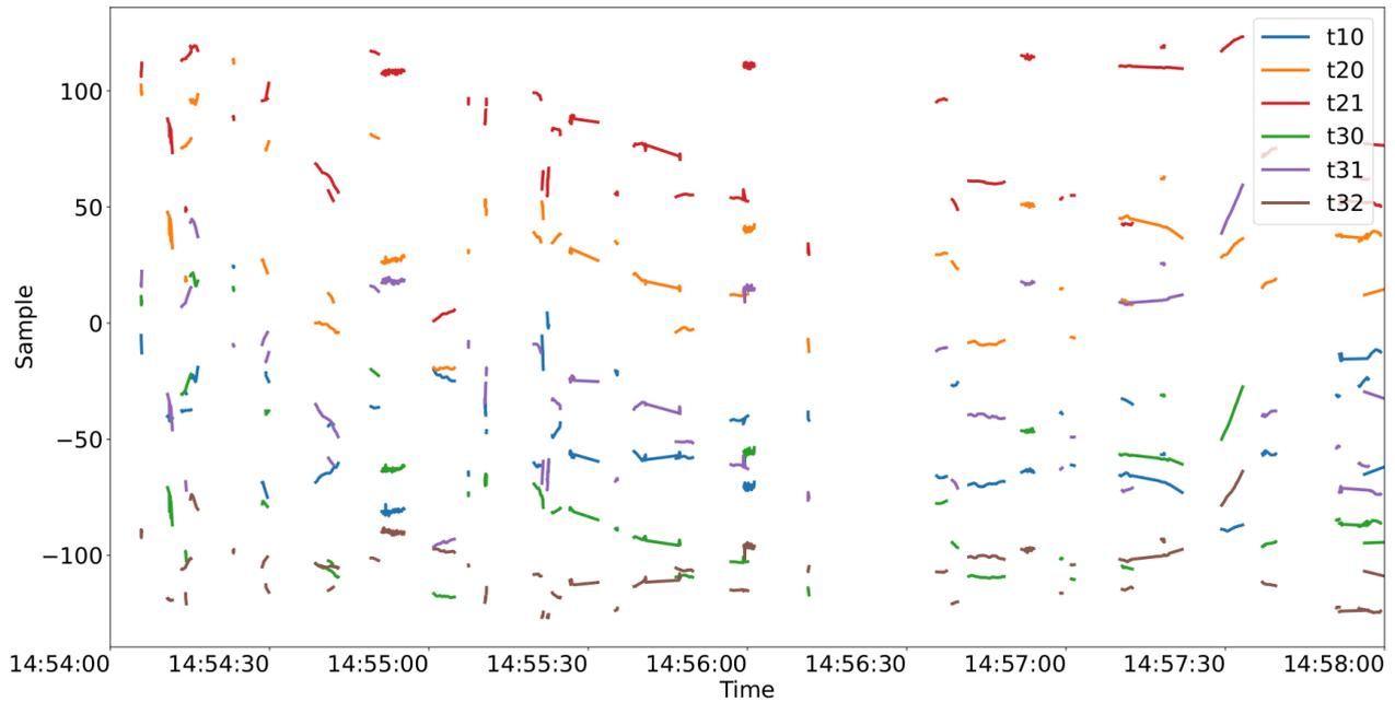
**Figure 5.16:** Example of delay time of arrival (TDoAs) in samples (Samples, 256 kHz Fe, ordinate) in 4 minutes of recording (abscissa) of orca clicks, for each pair of the 4 hydrophones of the Tetra antenna (t10, t20..). We can clearly see the TDoA tracks formed by a point source: the orca.
