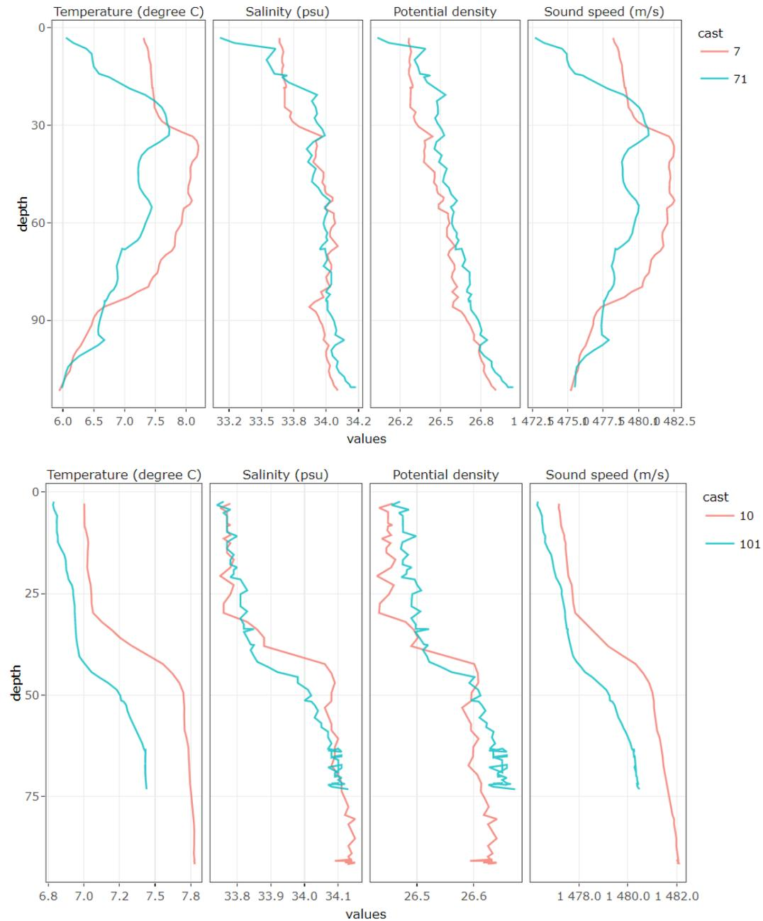
**Fig. 3.6 :** Comparison of CTD measurements before and after the gale of November 4-5, 2023: station 7 (before the gale) and 7bis noted "71" on the graph (after the gale), station 10 (before) and 10bis (noted 101 on the graph) (after the gale).
