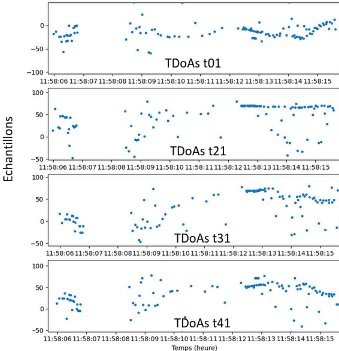
**Figure 7.15:** Example of delay time of arrival (TDoAs) in samples (256 kHz Fe, ordinate) in 8 seconds of recording (abscissa) of orca clicks, for each pair of the 5 hydrophones of the Opale antenna. We can clearly see the TDoA tracks formed by a point source: the orca.
