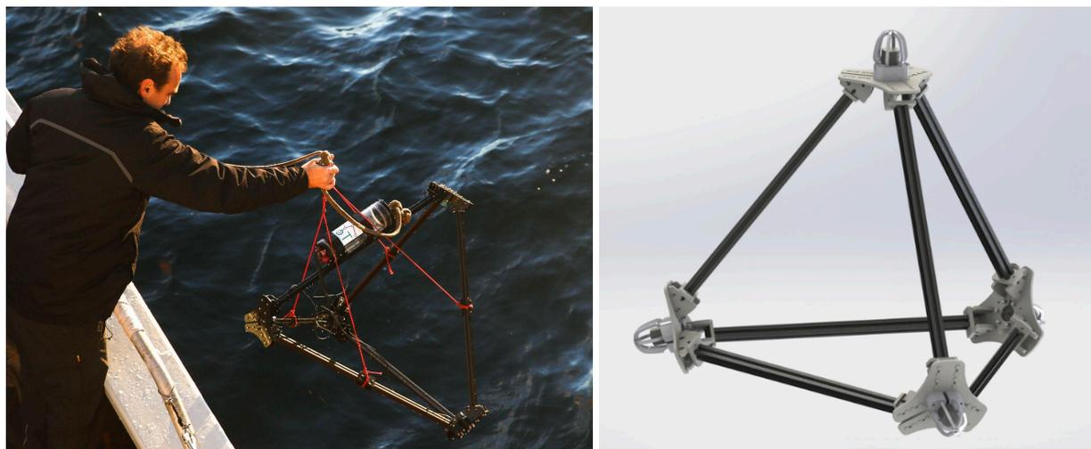
**Figure 4.4** : (Left) Launching from Isbjorn II (photo credit Gies) of the tetrahedral antenna, equipped with its sound card and four hydrophones, designed by SMIoT LIS IM2NP UTLN (Right).
