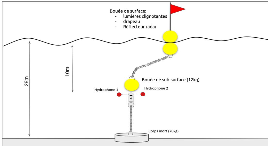
Figure 4.8 : Diagram representing the stereophonic buoy placed north of Haukøya. The mooring was designed by Dyni and Akvaplan-niva, the buoy instrumented by Dyni.
