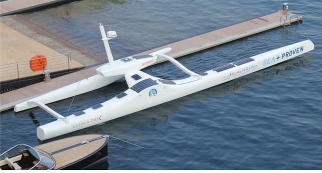
**Fig. 1.** The ASV Sphyrna, 17m long, Polynesian design.
