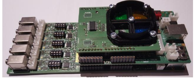
**Fig. 3.** The JASON sound card (SMIoT), 5 x 1 MHz sampling rate at 16 bits resolution, placed into the drone. The luxmeter was not used in this work.
