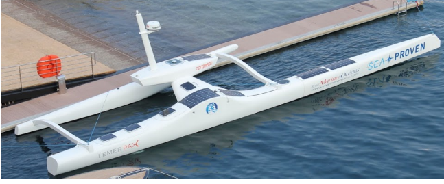
Fig. 1. The ASV Sphyrna, 17m long, Polynesian design.
