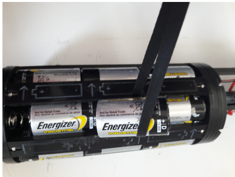
Ribbon on the last stack
